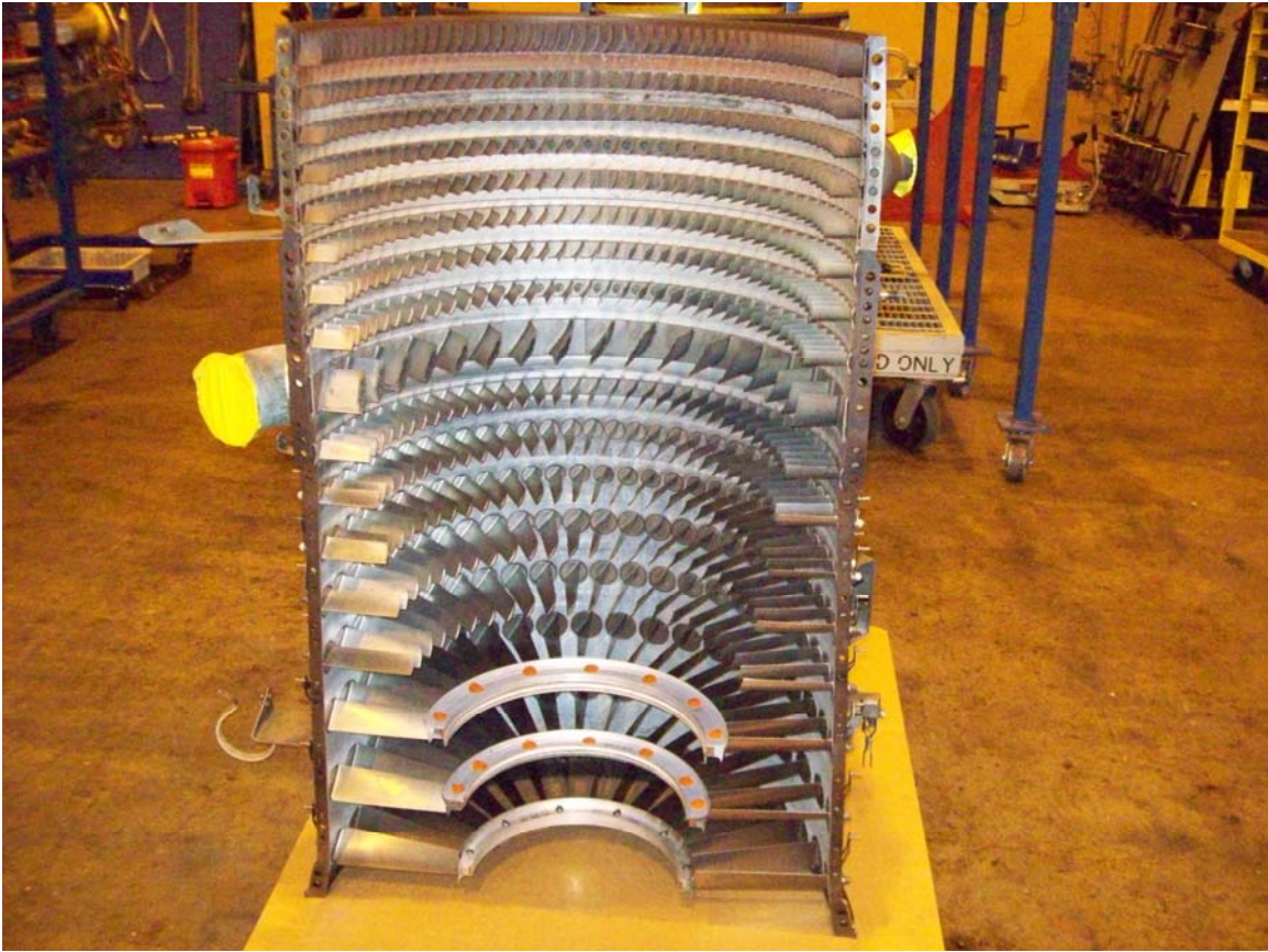
UPPER COMPRESSOR CASE AFTER REMOVAL
