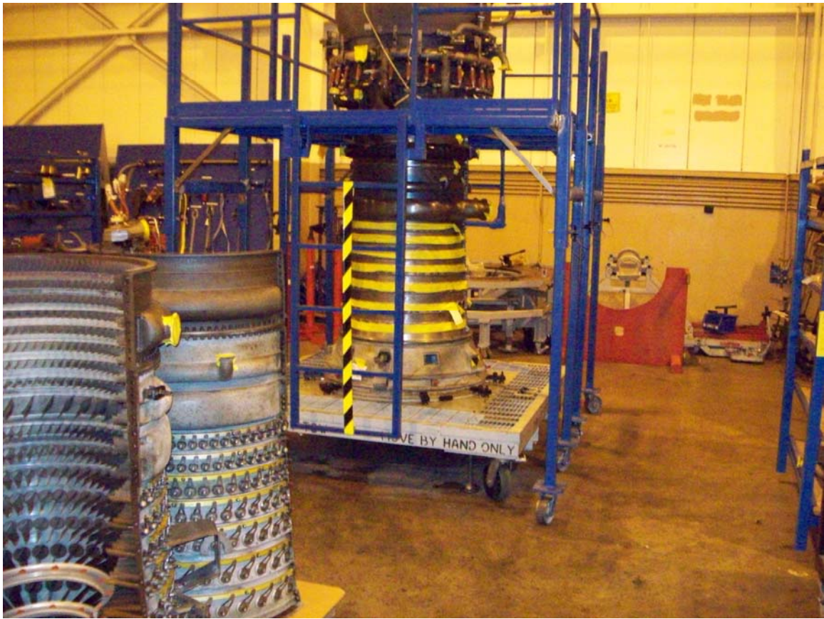
ENGINE VERTICAL WITH STABILIZER CASES FOR PROTECTION
