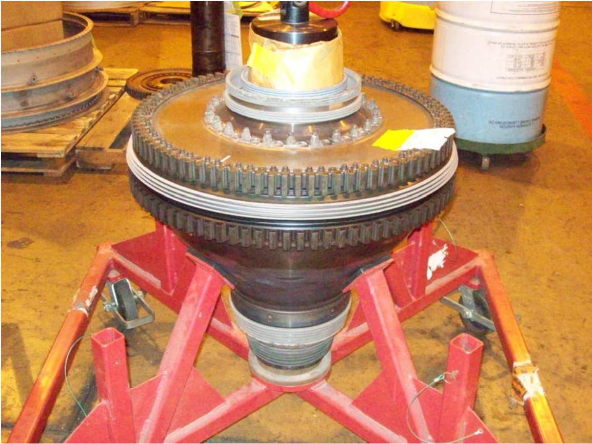
DEBLADED HPT ROTOR WAITING FOR BLADES TO COME BACK FROM REPAIR
